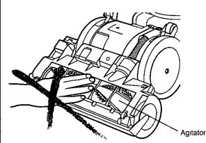
Iff it is necessary to remove threads, strings, hairs, etc., which have wound around the agitator, cut across them with a pair of scissors making sure not to cut the bristles
